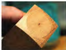
Shape now, drill later. Cut the pommel on the ends of the upper and lower sections, then drill out the mortise.
